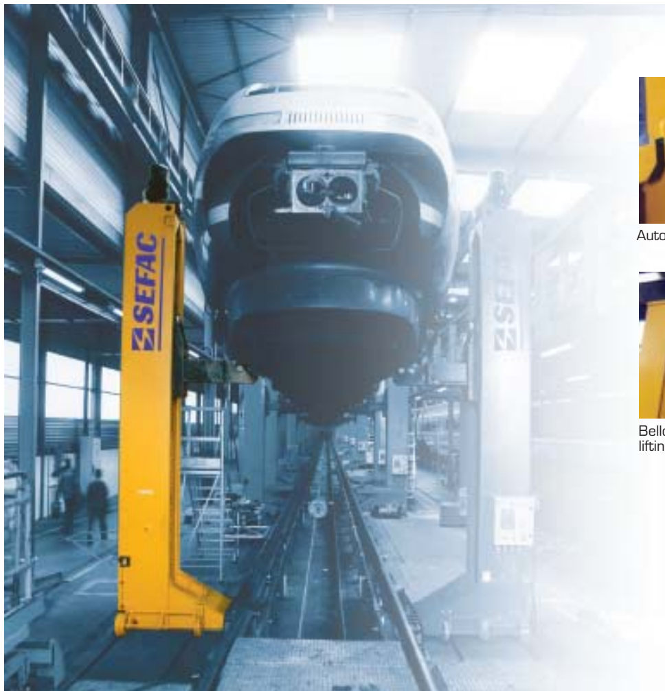
Motor geared column displacement system with foot protection.
